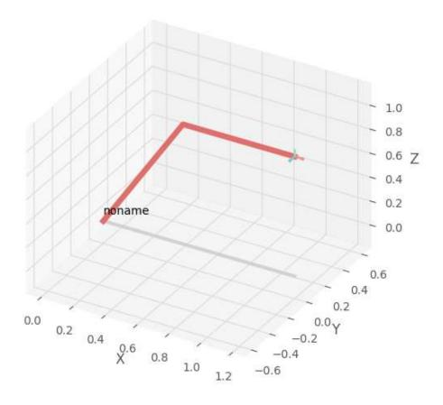
By giving an array of many elements as an argument to the **plot** method, it is possible to show an animation of the manipulator's movement.
